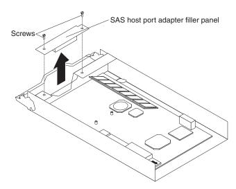
Figure 43. Removing the SAS host port adapter filler panel
